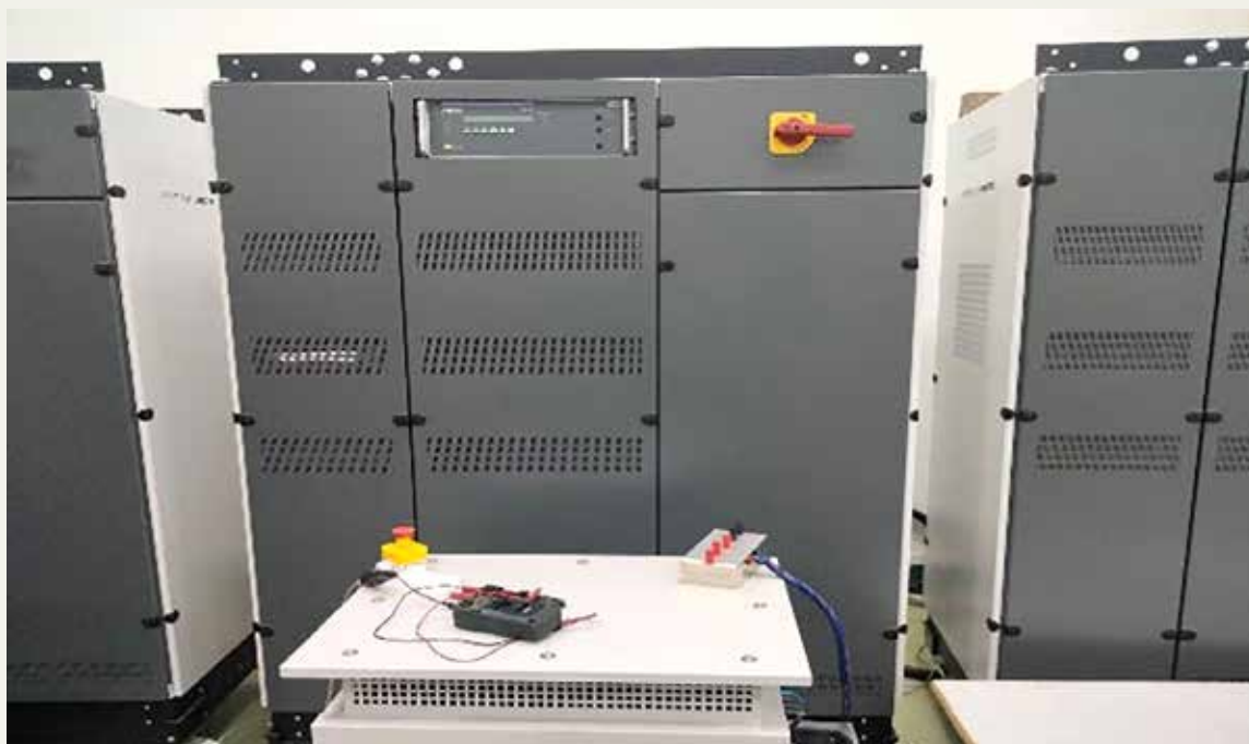
Test Setup for IEC 61000-2-2 (low frequency conducted disturbances)
